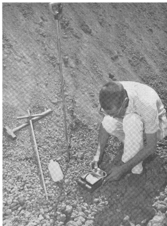
Measuring the electrical resistivity of a soil in the field .
