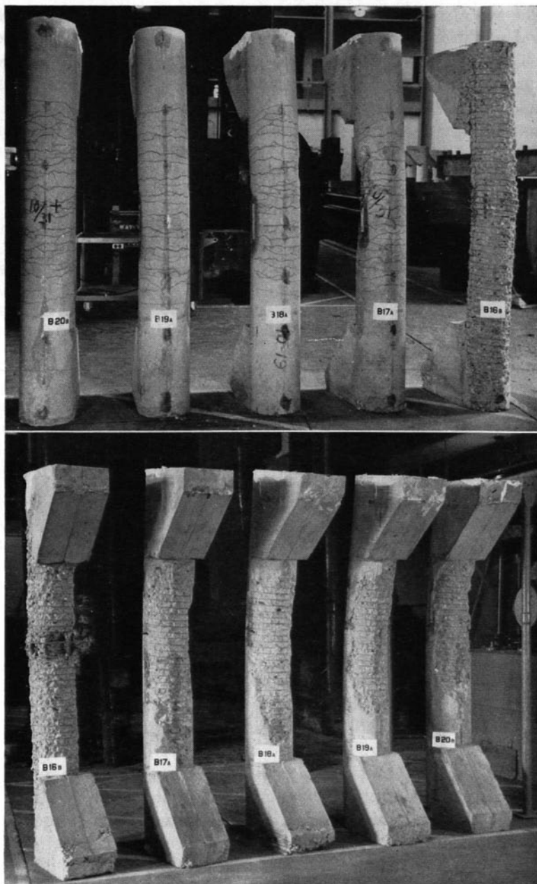
Fig. 39. Columns B-16 to B-20 after Failure
