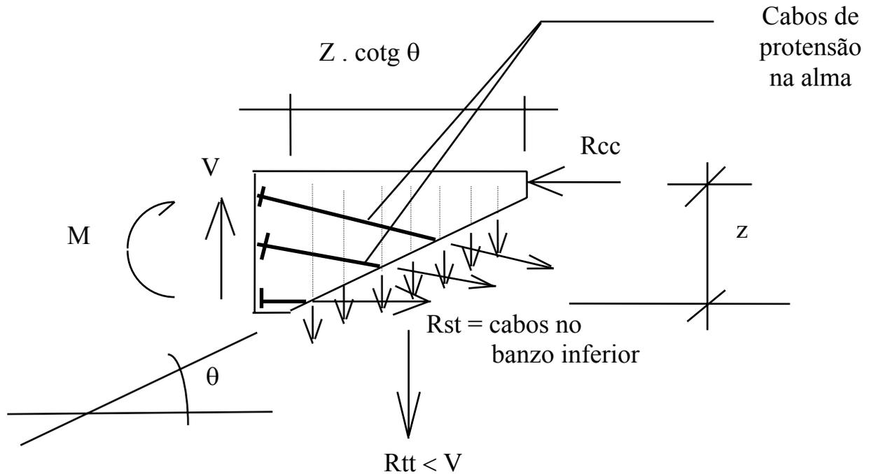
$$V = R_{tt} + \Sigma F \text{ cabos} \times \text{sen} \alpha$$
