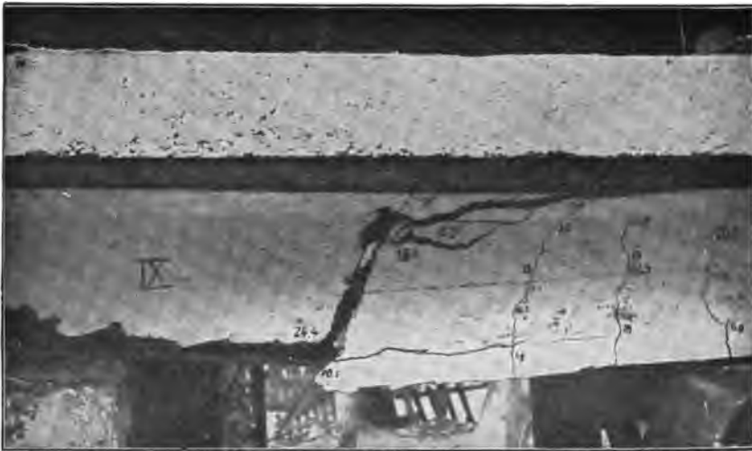
FIG. 156.—Beam IX, No. 2 rib, under the breaking load.
