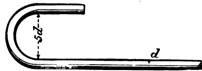
FIG. 127.—Form of hook, according to Considère.
