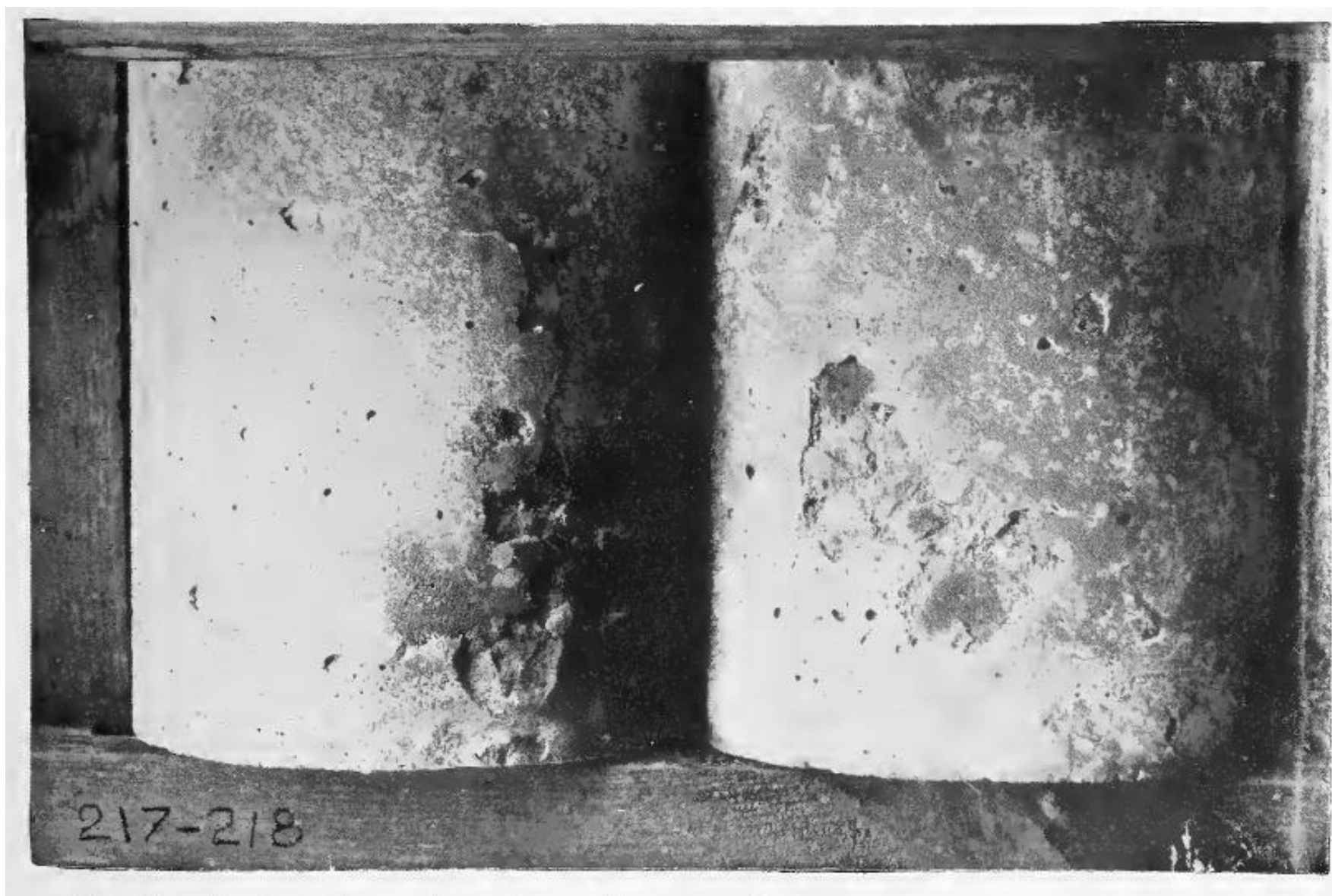
Fig. 25.—Portions of concrete specimens after one year's exposure to sea water, showing cracked surface and layer flaking off
