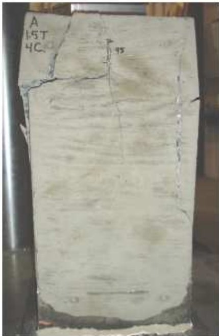
Figure 4-9: Failed Prisms with Tied Reinforcing
