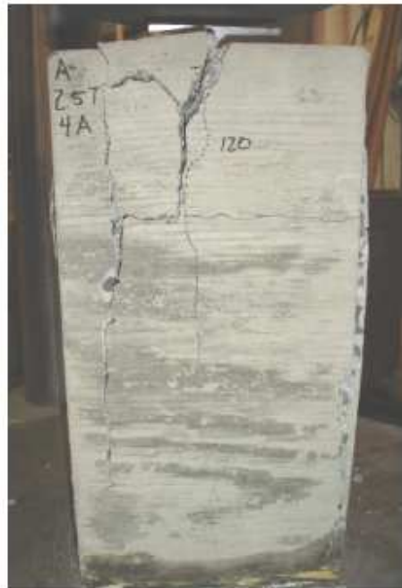
Figure 4-9: Failed Prisms with Tied Reinforcing
