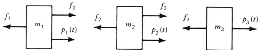
$$\begin{aligned} \sum F_x &= m_1 \ddot{u}_1 = p_1 + f_2 - f_1 \\ \sum F_x &= m_2 \ddot{u}_2 = p_2 + f_3 - f_2 \\ \sum F_x &= m_3 \ddot{u}_3 = p_3 - f_3 \end{aligned}$$
