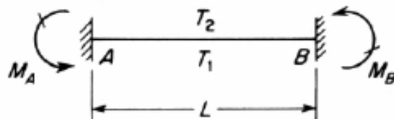
$$M_A = -M_B = \frac{\alpha EI(T_1 - T_2)}{d}$$
