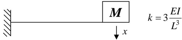
$$M = 40 \text{ kg} \quad m = 5 \text{ kg} \quad L = 1,0 \text{ m} \quad h = 1,0 \text{ m} \quad g = 10 \text{ m/s}^2 \quad EI = 1,5 \text{ kNm}^2 \quad L = 1 \text{ m}$$
