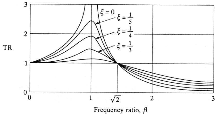
Vibration-transmissibility ratio (applied loading or support excitation).
