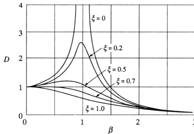
Variation of dynamic magnification factor with damping and frequency.
