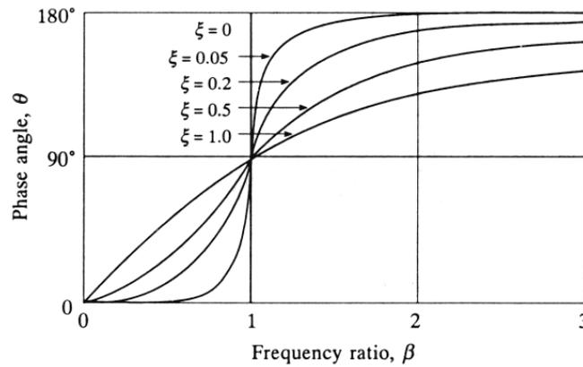
Variation of phase angle with damping and frequency.
