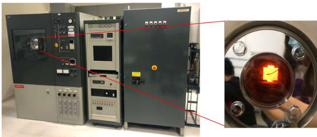
Figura 16 – Fluxograma do forno de "spark plasma sintering" (SPS).
