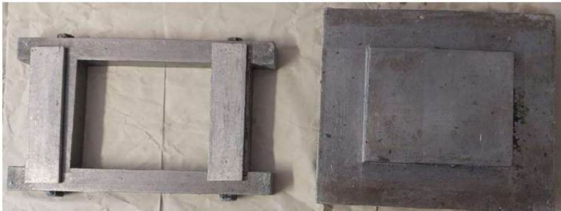
Figura 3.8 – Equipment that assisted in the manufacture of the composite plates, such as the parts that composed the steel matrix.
