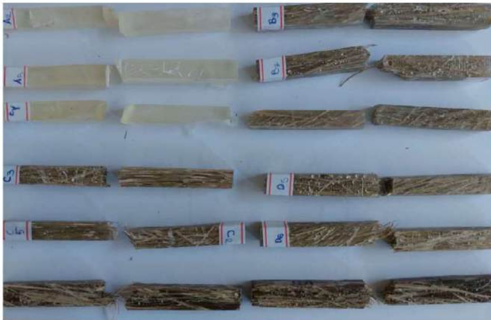
Figura 4.30 – Fracture of the samples 30 SF/EP-GO after the IZOD impact test.
