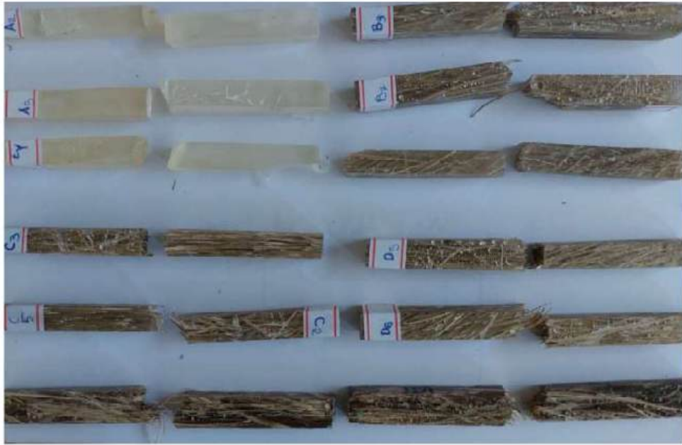
Figura 4.27 – Samples after the Charpy impact test.
