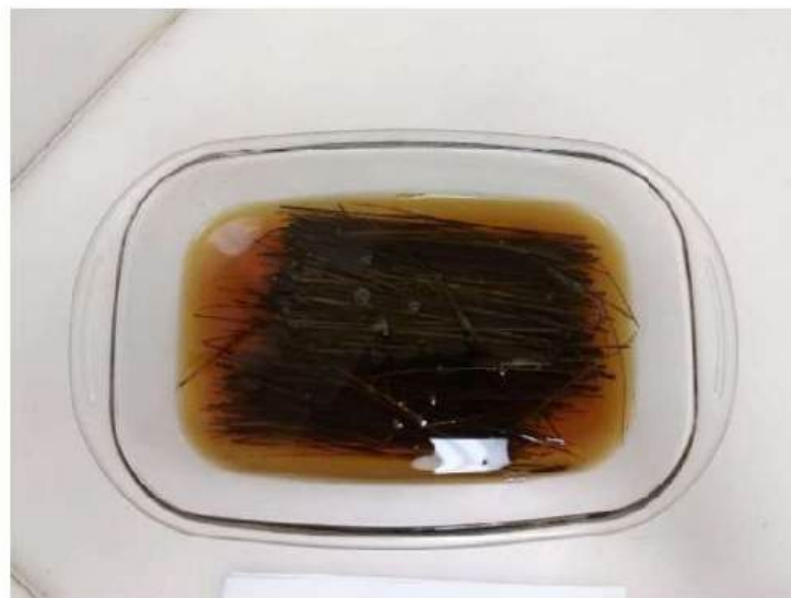
Figura 3.4 – Alkali treated fiber bundle after 24 h.
