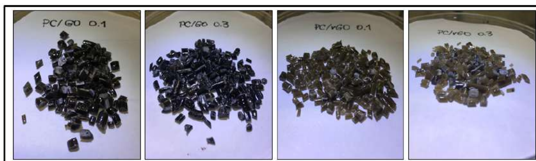
Figura 23 – Masterbatch dos nanocompósitos processados: PC/GO 0.1%, PC/GO 0.3%, PC/RGO 0.1% e PC/RGO 0.3%.
