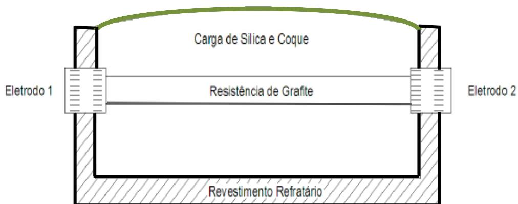
FIG. 2.10 Forno processo Acheson (GUPTA, 2001)
