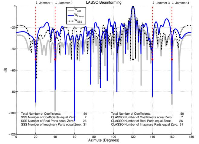
Figure 3. Beam pattern calculated for  $\theta = 120^\circ$ ,  $N = 50$ , and  $\alpha = 0.1$ .
