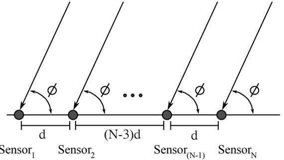
Figure 1. Narrowband Signal Model for Uniform Linear Array (ULA) for snapshot at instant  $t$ .
