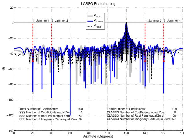
Figure 5. Beam pattern calculated for  $\theta = 120^\circ$ ,  $N = 100$ , and  $\alpha = 0.50$ .
