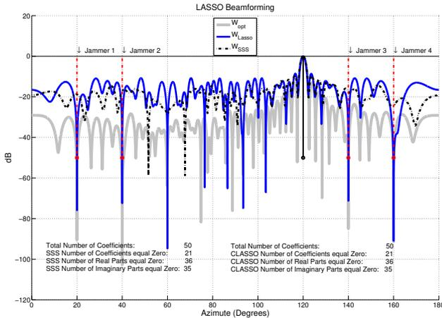
Figure 2. Beam pattern calculated for  $\theta = 120^\circ$ ,  $N = 50$ , and  $\alpha = 0.05$ .
