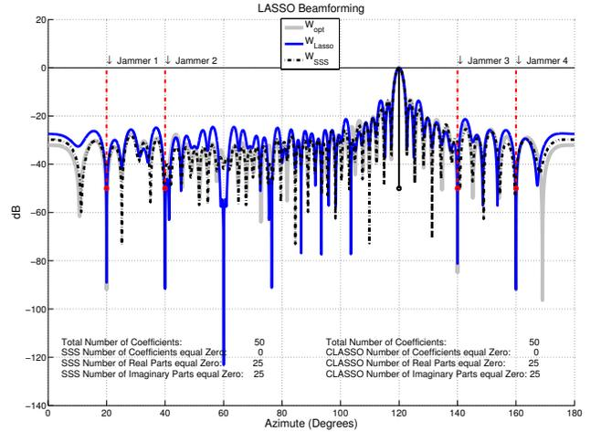
Figure 4. Beam pattern calculated for  $\theta = 120^\circ$ ,  $N = 50$ , and  $\alpha = 0.25$ .
