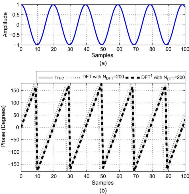
Fig. 2. Phase estimation of an artificial 60.98-Hz tone: (a) signal; (b) phase estimate.
