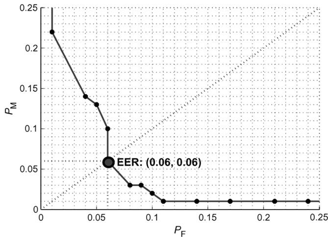
Fig. 6. DET curve:  $P_M$  versus  $P_F$  for the test audio *corpus*. The DFT<sup>1</sup>-based phase estimation method was used, with a window size of 10 cycles of the nominal ENF and  $N_{\text{DFT}} = 2000$  points.
