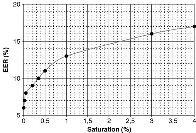
Fig. 12. Effect of saturation: EER in the task of audio authentication as a function of the saturation level. The system error without artificial nonlinearity is 6%.
