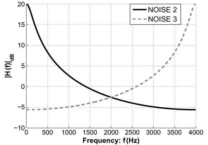
Fig. 9. Frequency response curves corresponding to  $H_{\text{LP}}(z)$  and  $H_{\text{HP}}(z)$  for NOISE 2 and NOISE 3, respectively. The curves were plotted as a function of the frequency  $f$ , in hertz, assuming a sampling rate of 8000 Hz.
