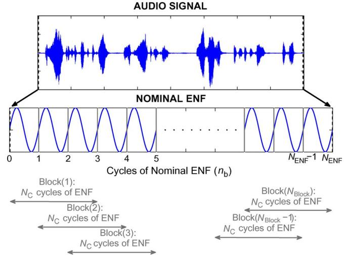
Fig. 3. Block fragmentation of an audio signal.  $N_{ENF}$  is the number of ENF cycles in the audio signal;  $N_{Block}$  is the number of fragment blocks;  $N_C$  is the number of ENF cycles in each block.
