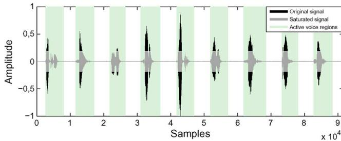
Fig. 11. Example of a signal with 3% saturation level, i.e., with 3% of the samples in active (shaded) regions clipped to a maximum level.
