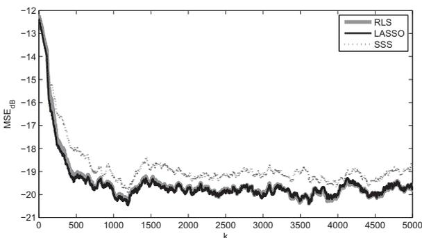
Fig. 8. Learning curves for the ITU-T G.168 echo path identification experiment.
