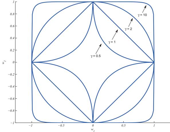
Fig. 3. Boundaries of the constraint sets for different values of  $\gamma$  [2].
