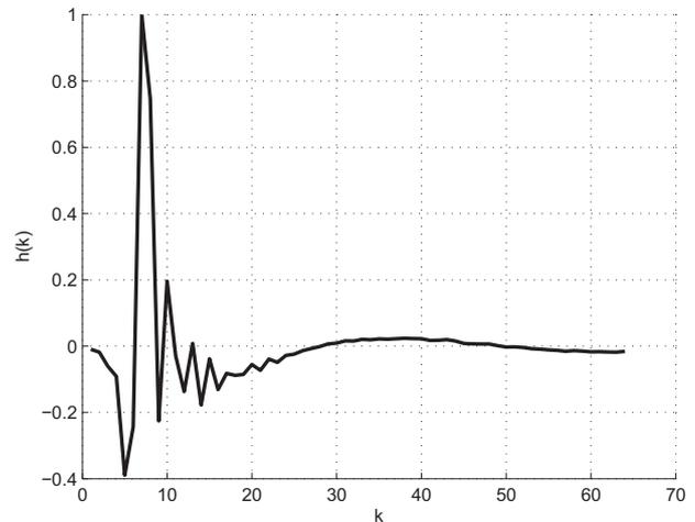
Fig. 6. Impulse response of the ITU-T G. 168 echo path model 1.
