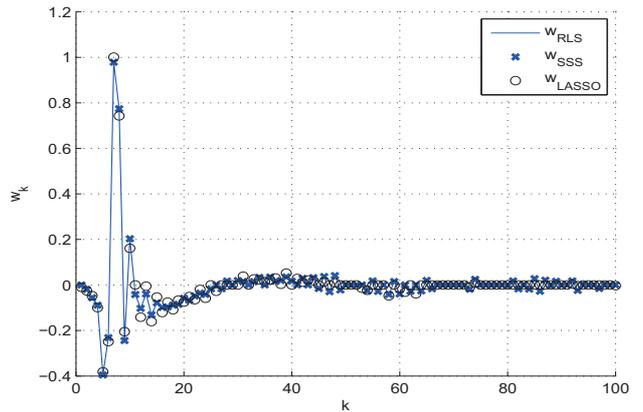
Fig. 9. Adaptive filters regressors for the sparse system identification experiment.
