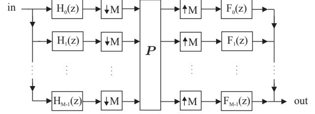
Fig. 1. Block diagram of a Frequency Domain Scrambler.
