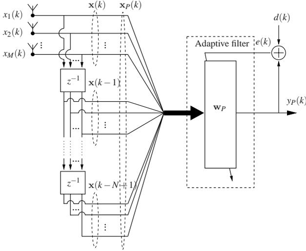
Figure 1: Multichannel adaptive filter setup.
