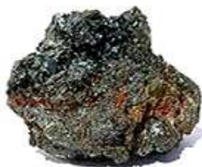
Hematita preta \equiv \text{Fe}_2\text{O}_3
